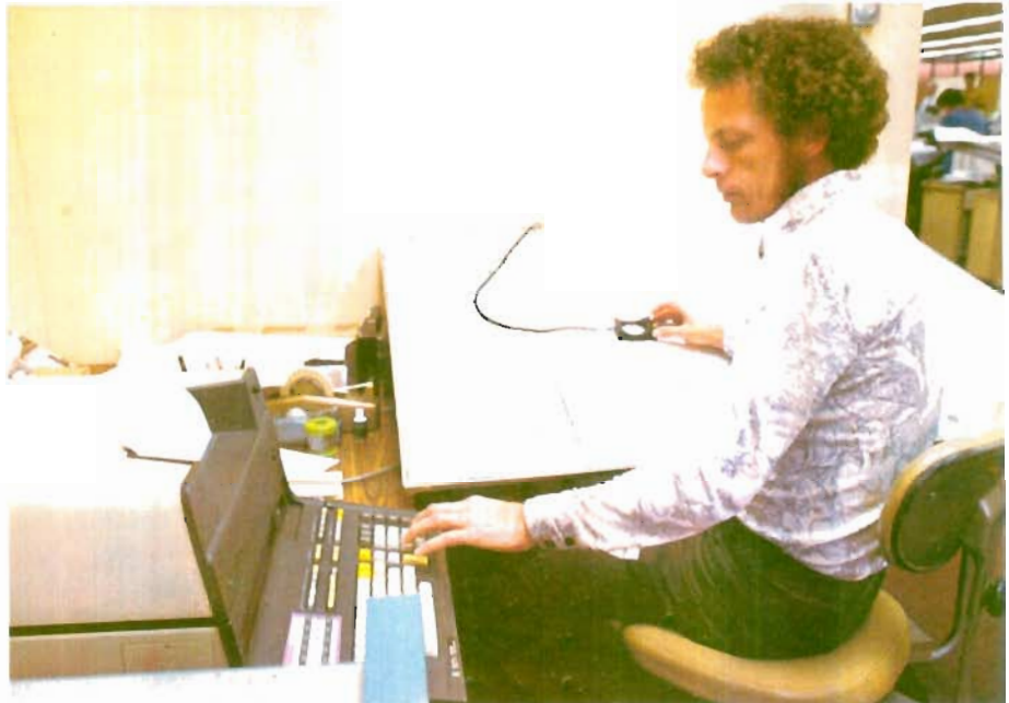
Computer graphics system with digitizer in typical application, determining length of pipe in network
