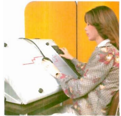
The HP 9874A Digitizer assists in printed-circuit layout.
