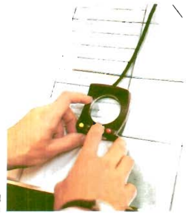
Data tablet speeds entering of data selected from several alternatives.
