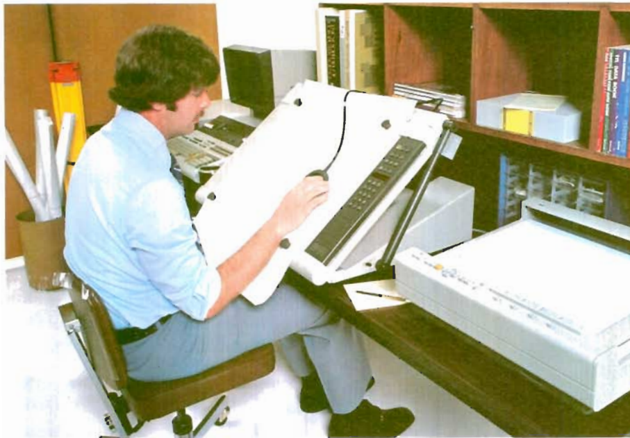
Computer system with 9874A Digitizer enhances mapping and area measurements.
